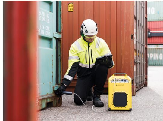
The Calcmet software includes indicators of danger or unknown compounds. In the case of indications of interference from unexpected gases, Calcmet provides automatic search tools for identifying unknown gases with just a few easy steps, and once identified, new components can be added to the list of measured compounds for quantification.
