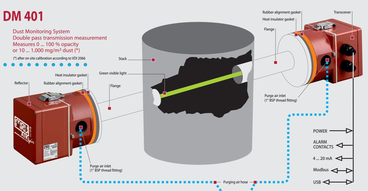
DM 401 is the ideal dust monitoring instrument for continuous monitoring of flue gas particulates in the ducts / stacks / chimneys of industrial combustion.
